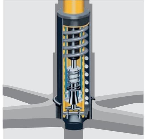
**Sedo-Lift mechanism.** Even in the lowest position, this seat-height adjustment – with worldwide patent – provides a back-friendly “soft landing” when you sit down. Grooves have been cut into the side of the guide tube, into which the mechanism clicks into place. This takes the pressure off the gas lift mechanism, which is why it is so durable. Sedus provides a 30-year guarantee!
